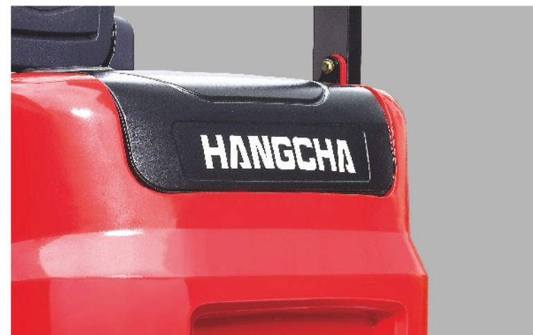
Easy opened counterweight cover is to protect the internal controllers to avoid water and dust.
