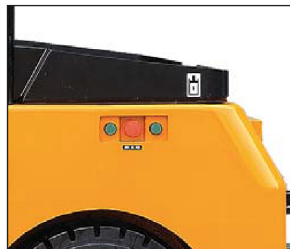
Forward/Reverse inching switch and emergency stop button are mounted on the left rear, they make the hook easy and safe.
