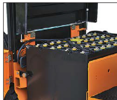
The battery cover can be fully opened, the design is easy for maintenance.
